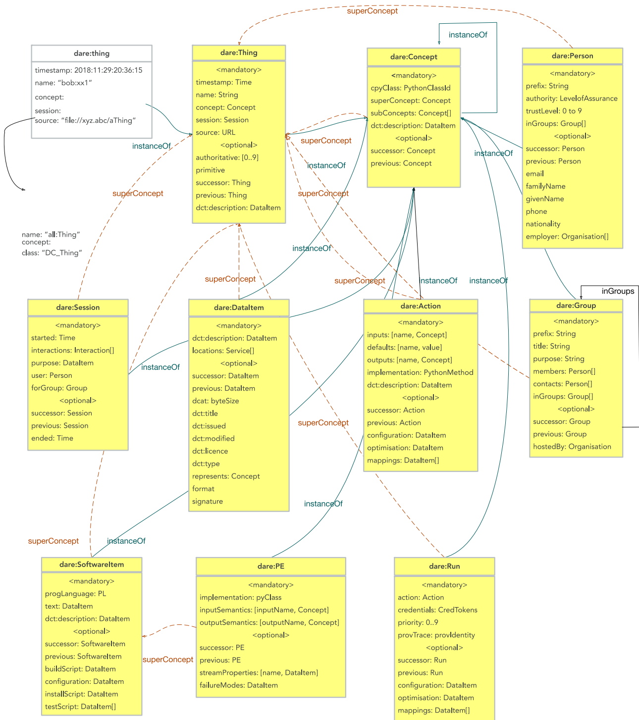
Figure 12: The DARE core Concepts. One instance of Thing is shown in white. Instances of Concept are shown in yellow. The arcs illustrate some relationships; not all are shown.
